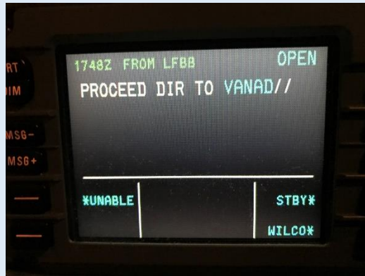
Figure 6: CPDLC PROCEED DIRECT received by LFBB displayed on an Airbus DFU
