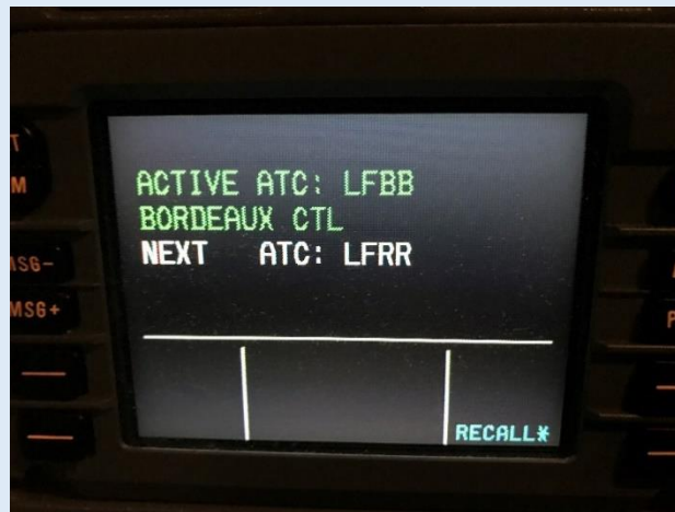
Figure 3: Current Data Authority (CDA) along with Next Data Authority (NDA) displayed in Airbus DFU displays
